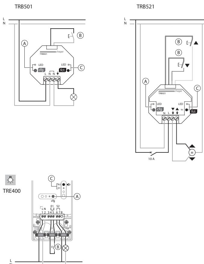
A Button and LED configuration "cfg"
