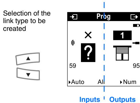
The « symbol indicates that it is a radio input. To select the functions, switch to the numbering mode.
