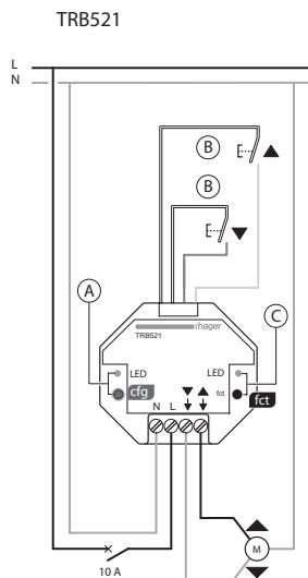
A Button and LED configuration "cfg"
