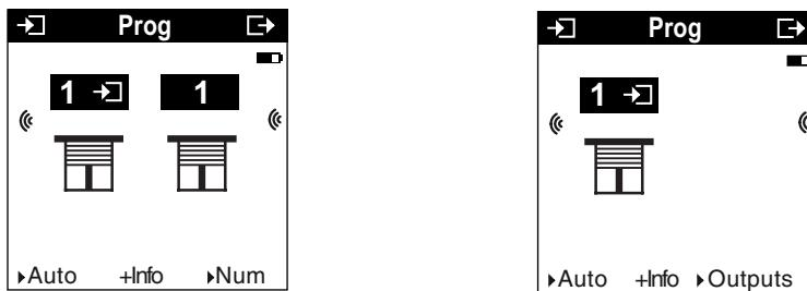
The +Info mode allows the status indication to be linked from an output to a viewing product: Area controller, LED output, etc. The status indication sends the current status over the network each time the status changes.
