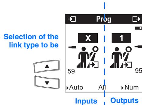
Link creation is used to connect the master detector and the slave detector.
